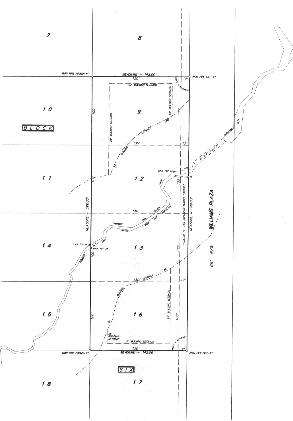
NOTE: SURVEYOR'S ORDINARY HIGH WATER MARK = TOP OF BANK D.N.R. FLAGGING (TOP OF BANK) DATED AND MARKED 4/21/04 E. KING
